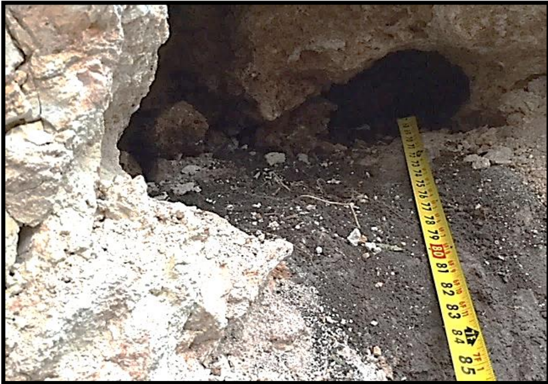
Photo 9. Feature S-8 maximum horizontal extent (approximately 7 feet) of the horizontal solution cavity along the long axis.
