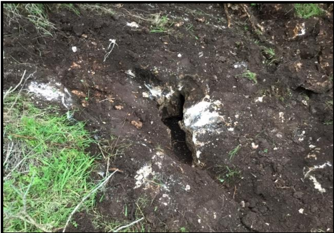
Photo 2. Top of limestone bedding unit at Feature S-7 following removal of soil and vegetation.
